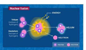
• Process: The Deuterium (H-2) and Tritium (H-3) atoms are combined to form Helium (He-4). A free and fast neutron is also released as a result.
